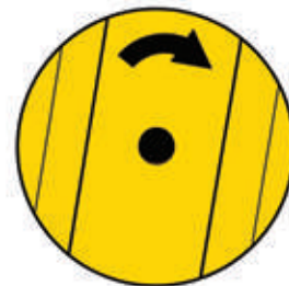
The right way to roll the drums Follow the direction shown by the arrow
